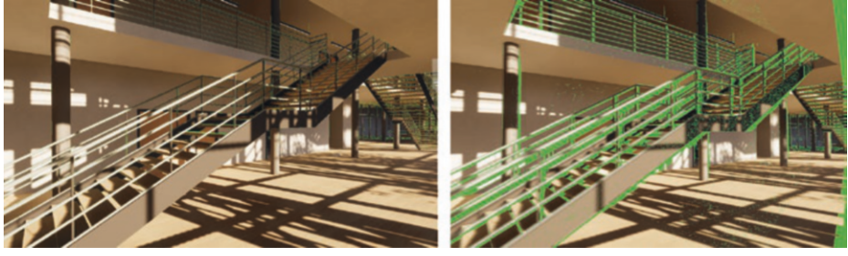
Figure 26-5. This image highlights the areas where a new diffuse ray is requested (green). Left: the camera is stationary. Due to the temporal antialiasing camera subpixel offset, the reprojection fails at geometry edges. Right: the camera is moving to the right. New rays are requested at geometric occlusions and areas that were not present in the previous view. Note the partially green walls due to a decrease in the density of accumulated samples.
