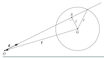
**Figure 7-5.** Geometric setting for options to compute  $l^2$ . The ray origin 0, the sphere center G, and its projection, S, onto the ray form a right-angled triangle.
