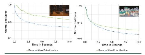
**Figure 23-16.** Convergence plots for demonstrating performance gain by using view prioritization on two scenes: Granary by Night (left) and Zen Peak (right). These plots show the error (L1) compared to a reference light map. View prioritization (dashed curve) allows for faster convergence, especially during the first few seconds, compared to scheduling all light map texels at once (red curve).
