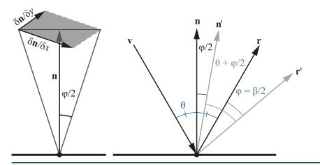
**Figure 20-7.** Left: the geometry involved in computing  $\phi$ . Right: the view vector **v** is reflected around the normal **n**, which generates **r**. If **n** is perturbed by  $\phi/2$  into **n**', we get another reflection vector **r**'. Since  $[-\mathbf{v}, \mathbf{n}'] = \theta + \phi/2$ , we have  $[\mathbf{r}', \mathbf{n}'] = \theta + \phi/2$ , which means that the angle  $[\mathbf{r}, \mathbf{r}'] = \phi$ , i.e., is twice as large as  $[\mathbf{n}, \mathbf{n}'] = \phi/2$ .
