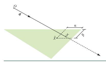
**Figure 6-2.** Calculating the intersection X with barycentric coordinates  $(\alpha, \beta)$ . In this case, the finite precision of  $(\alpha, \beta)$  means that the computed intersection point  $\tilde{X}$  may no longer lie exactly on the ray—but it will always be very close to the surface.
