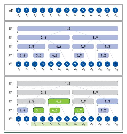
**Figure 5-2.** Illustration of the recursive range tree method. Given input array A (top), we compute a binary tree (middle) where each node stores the minimum and maximum of its corresponding leaf nodes. Our recursive traversal for a query range (bottom) uses all three cases from the pseudocode: gray nodes recurse into both children (case 3), green nodes with dark outlines get counted and terminate (case 2), and blue nodes with dashed outlines lie outside the range (case 1).
