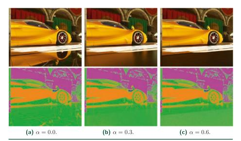
**Figure 32-13.** Varying the material roughness ( $\alpha$ ) of the floor, with reflections maps at the bottom. As the material gets rougher, more samples are fetched from the cache or fully shaded as they deviate from screen space: this can be seen at the bottom of the mask as the color turns from dark green to light green and orange. Mirror-like surfaces sample effectively from screen space when possible.
