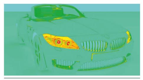
**Figure 10-3.** Heat map of the approximate per-pixel cost of the scene shown in Figure 10-1. The palette of the heat map is (from low to high cost) turquoise, green, yellow, orange, red, and white.
