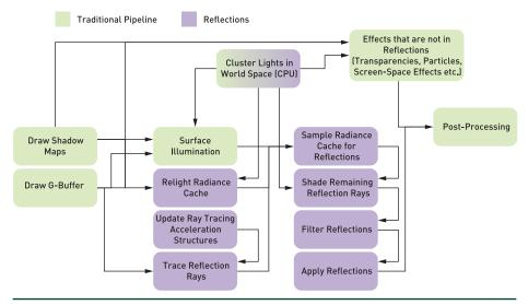
Figure 32-2. Stages and data flows of the overall rendering pipeline and their dependencies.
