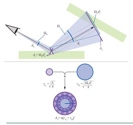
**Figure 31-4.** Our footprint heuristic. Due to BSDF scattering the solid angle grows with each interaction  $(\Omega_1 > \Omega_0)$ . The footprint size depends on the previous area as well as  $\Omega d^2$  for the new scattering. The combination of the two areas is achieved by a convolution (bottom).
