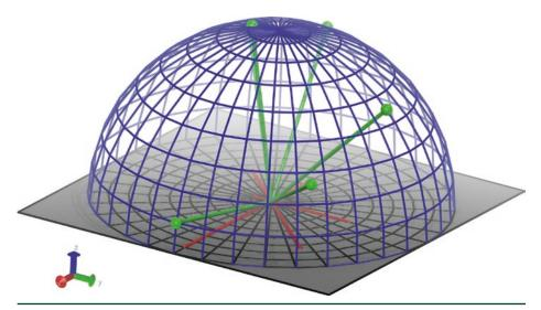
**Figure 4-2.** A visual depiction relating the image plane (gray square with inscribed latitude/longitude lines), dome hemisphere (blue), example **p** vectors (red) in the image plane, and corresponding ray directions on the dome surface (green).
