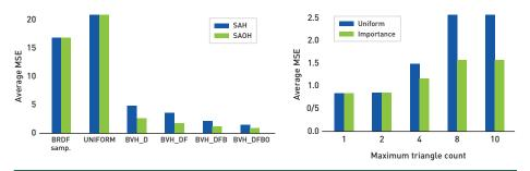
**Figure 18-8.** Comparisons in Bistro (view 3) of mean squared error (MSE) results for the different traversal methods, compared to sampling the BRDF to get the light sample direction (left) and various maximum amounts of triangles for BVH\_DFB0 (right). All methods use 4 samples per pixel, and BVH-based methods use 16 bins along all three axes.
