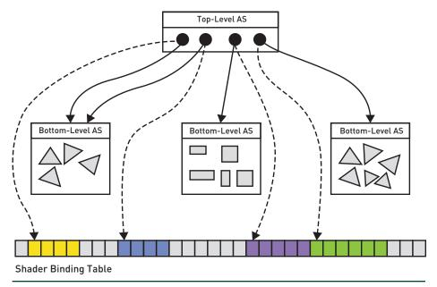
Figure 19-1. The two-level hierarchy of the acceleration structure.
