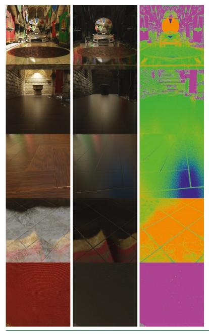
**Figure 32-10.** Test cases from top to bottom: Main, Spot, Wood, Tile, and Curtain.Left: the final illumination. Center: the environment reflection term. Right: the reflection mask (color map as described in Section 32.5). These images were captured from a static camera for a static scene.
