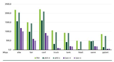
**Figure 9-3.** Performance of standard first-hit and multi-hit variants for finding first intersection. The graph compares performance in millions of hits per second (Mhps) among standard first-hit traversal and our multi-hit implementations when  $N_{avery} = 1$ .
