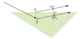
**Figure 6-5.** Setting  $t_{min}$  to a small value  $\varepsilon > 0$  does not robustly avoid self-intersection, especially for rays exiting at grazing angles. In the example the distance t along the ray is greater than  $t_{min}$ , but the distance  $\delta$  of the (false) next intersection  $\tilde{X}'$  to the surface is zero due to finite precision.
