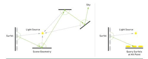
Figure 25-30. Left: full recursive path tracing. Right: incremental previous frame path tracing.
