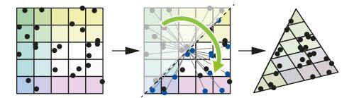
To avoid the square root, you can also sample from a quadrilateral and flip the sample if you are on wrong side of the diagonal. However, flipping over the diagonal can reduce the effectiveness of blue noise or low-discrepancy sampling within the triangle, as there is usually no guarantee that well-distributed points in two dimensions remain well distributed when folded.
