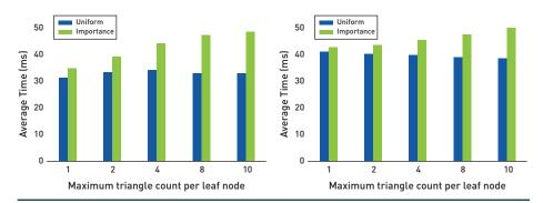
**Figure 18-5.** Rendering times in milliseconds per frame for various maximum numbers of triangles per leaf node for Bistro (view 1) (left) and PBG-R (right), with and without importance sampling for triangle selection within the leaves. In all cases the BVH was built with 16 bins along all three axes using SAOH, and BVH\_DFBO was used for the traversal.
