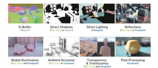
Figure 25-2. Hybrid rendering pipeline.
