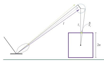
**Figure 32-5.** Thresholds used for radiance probe sampling: visualization of the resolution threshold heuristic. The value  $\frac{n}{x_c}$  is half a pixel in width in world space at the cube map's near plane at distance n. This value is then proportional to the radius of the circle sampled at  $z_c$ .
