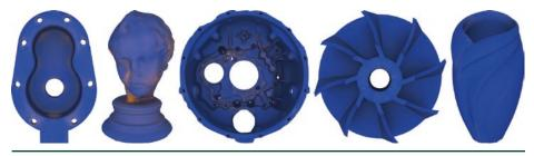
**Figure 8-6.** Color-coded errors in models from Fang et al. [9] collection. We linearly interpolate from blue (for error = 0) to brown (for error  $\geq 10^{-5}$ ).
