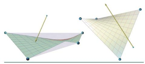
**Figure 8-5.** Left: ray intersects planar patch at  $\{u, v\} = \{0.3, 0.5\}$  and  $\{0.74, 2.66\}$ . Right: there is no intersection between the ray and the (extended) bilinear surface in which the patch lies.
