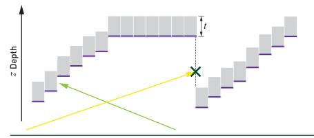
**Figure 26-3.** Ray traversal in screen space. The front layer depth of the Z-buffer (purple line segments) is assumed to have a thickness t. This helps to prevent rays from penetrating closed surfaces (green ray). To minimize errors, we discard a screen-space ray when it enters areas behind the assumed thickness of the front layer (yellow ray) and continue tracing it in the BVH.
