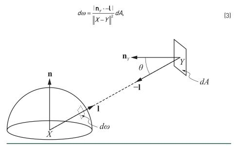
**Figure 18-2.** The differential solid angle  $d\omega$  of a surface patch dA at a point Y on a light source is a function of its distance ||X - Y|| and the angle  $\cos\theta = |\mathbf{n}_Y \cdot -\mathbf{l}|$  at which it is viewed.
