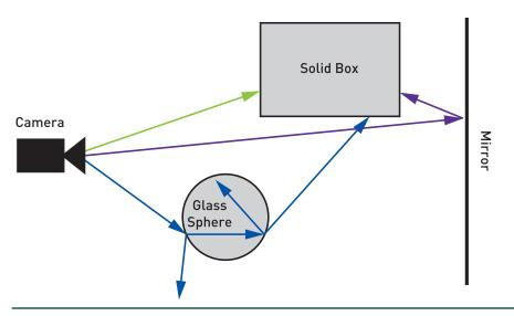
**Figure 1-2.** Ray tracing. Three rays travel from the camera into the scene. The top, green ray directly hits a box. The middle, purple ray hits a mirror and reflects to pick up the back of the box. The bottom, blue ray hits a glass sphere, spawning reflection and refraction rays. The refraction ray in turn generates two more child rays, with the one traveling through the glass spawning two more.
