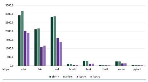
**Figure 9-4.** Performance of multi-hit variants for finding all intersections. The graph compares performance in Mhps among our naive and node-culling variants when  $N_{query} = \infty$ .
