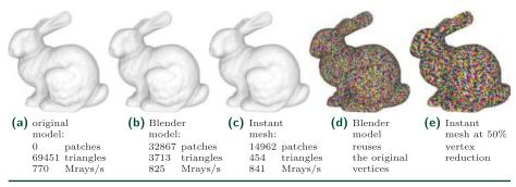
Figure 8-3. Different versions of the Stanford bunny ray traced on a Titan Xp using ambient occlusion.
