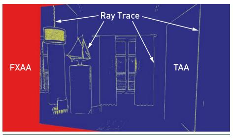
**Figure 22-3.** An annotated visualization of an ATAA segmentation mask. Blue pixels use standard TAA, red pixels use FXAA, and yellow pixels use ray traced supersampling.
