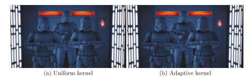
**Figure 19-15.** Indirect lighting filtered with (a) a uniform world-space radius and (b) an adaptive kernel. The adaptive kernel size is based on average ray hit distance and accumulated temporal sample count.
