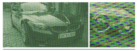
**Figure 10-2.** Adaptive tiling for four processing units with relative weights of 10% (red), 15% (yellow), 25% (blue), and 50% (green). Note how the headlight pixels are distributed among processing units.
