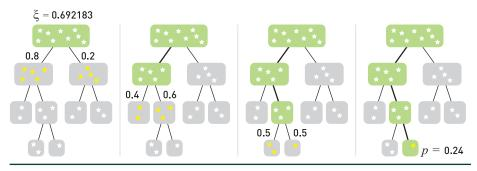
**Figure 18-1.** All the light sources in the scene are organized in a hierarchy. Given a shading point X, we start at the root and proceed down the hierarchy. At each level, the importance of each immediate child with respect to X is estimated by a probability. Then, a uniform random number  $\xi$  decides the path through the tree, and at the leaf we find which light to sample. In the end, more important lights have a higher probability of being sampled.
