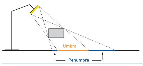
**Figure 1-3.** An area light casts a soft penumbra shadow region, with the umbra being fully in shadow.
