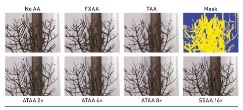
**Figure 22-8.** Zoomed images from the Modern House scene highlighting a challenging area featuring complex detail from a plant, comparing plant details rendered with 1 SPP rasterization, FXAA, UE4's stock TAA, a visualization of our segmentation mask, ATAA 2×, 4×, and 8×, and an SSAA 16× reference.
