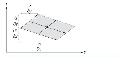
**Figure 20-1.** The footprint of a pixel approximated as a parallelogram in texture space. This notation is used in Equation 2.
