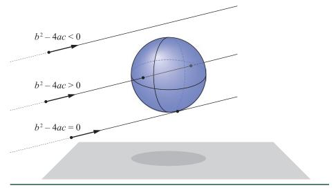
**Figure 7-2.** Ray/sphere intersection test. The three different types of intersections are, from top to bottom, no hit, two intersection points, and a single hit (when the two intersections are the same).
