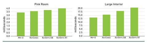
**Figure 20-12.** Performance impact of texture level of detail selection methods: Pink Room (left) and Large Interior (right). The smaller scene (Pink Room) is less susceptible to an extra filtering cost, the larger scene (Large Interior) more so.For both scenes, however, the performance impact of RayDiffs GB is about 2×, and RayDiffs RT about 3×, the impact of RayCones.
