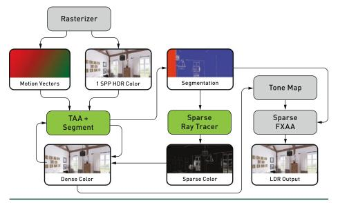
**Figure 22-2.** The data flow of ATAA integrated into the UE4 rendering pipeline. Gray boxes represent operations that are either unchanged or slightly modified. Green boxes represent operations that are modified or new. The Segmentation and Sparse Color buffers are new.
