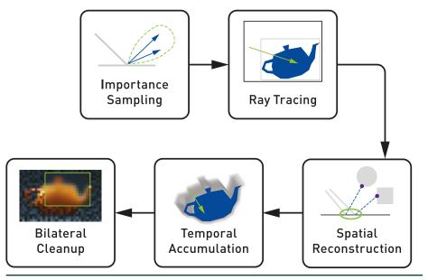
Figure 25-10. Reflection pipeline.
