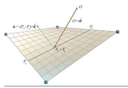
Figure 8-4. Finding ray/patch intersections.
