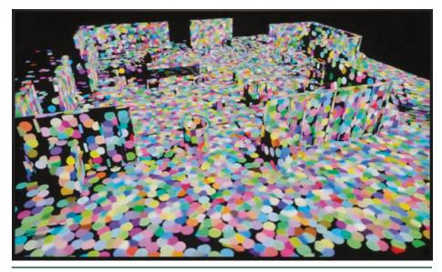
Figure 25-27. Surfels progressively allocated to the scene.
