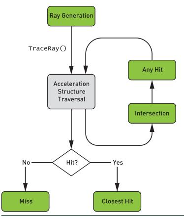
Figure 19-2. The ray tracing pipeline.
