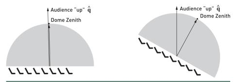
**Figure 4-4.** Relation between the dome zenith and audience "up" direction  $\hat{q}$  in both a traditional flat planetarium dome (left) and a more modern dome theater with 30 tilt and stadium style seating (right).
