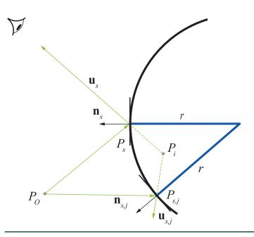
Figure 32-8. Reflection from a spherical mirror.
