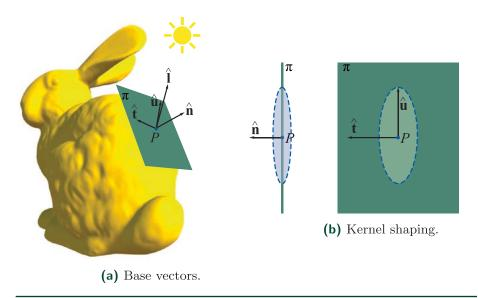
**Figure 24-4.** Left: the base vectors for the kernel space:  $\omega_g$  is aligned to the photon normal  $\hat{\boldsymbol{n}}$ , which also defines the kernel plane  $\pi$ . Two other basis vectors lie in  $\pi$  such that  $\hat{\boldsymbol{u}}$  is the projection of light direction  $\omega_i$  on to the kernel plane and  $\hat{\boldsymbol{t}}$  is orthogonal to  $\hat{\boldsymbol{u}}$ . Right: the kernel's shape is modified by scaling along those vectors.
