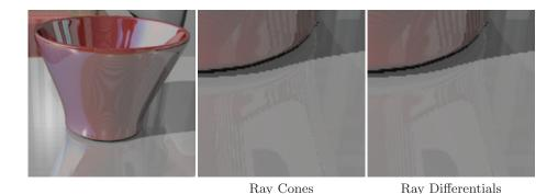
**Figure 20-8.** Zooming in on the base of a vase reflected in a table top shows that the ray cones method is weaker than the method based on ray differentials in areas of recursive reflections. In the lower part of the ray cones image, there is a substantial amount of aliasing, which is caused by the fact that, in our implementation, the method assumes that all surfaces beyond the first hit are planar.
