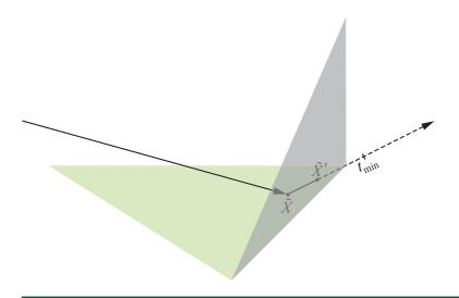
**Figure 6-6.** Skipping over a valid intersection  $\hat{X}'$  due to setting  $t_{min} = \varepsilon > 0$  is especially visible in corners due to paths being pushed into or out of closed objects.
