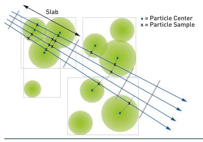
**Figure 29-2.** Overview of our algorithm. The geometric primitive is a spherical radial basis function centered at a point. The hit position is the distance to the particle center evaluated along the view ray. To ensure coherent behavior during traversal of this geometry, we divide the volume into segments along rays, resulting in slabs. We then traverse and sort the set of intersected particles within each slab.
