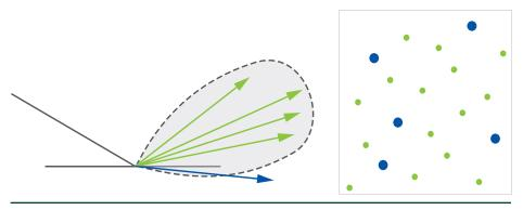
**Figure 25-11.** Left: BRDF reflection sampling. Right: Cranley-Patterson rotated Halton sequence. The probability distribution (light gray area with dashed outline) contains valid BRDF importance-sampled reflection rays (green) and reflection rays below the horizon (blue).
