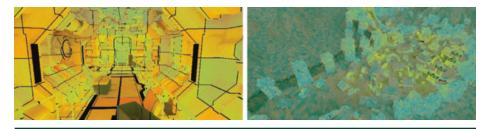
**Figure 23-12.** Number of local light queries per texel: blue is none, orange is most dense. Left: many local lights in a corridor. Right: sparse distribution of local lights with some hash collisions in an outdoor environment.
