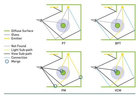
**Figure 31-1.** Visualization of paths that are found and not found by different methods. The area and the point lights at the ceiling cause different challenging light effects.
