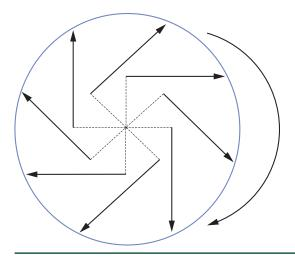
**Figure 4-5.** Illustration of the circular stereoscopic projection technique and the effect of applying an eye offset of half of the interocular distance to each ray's origin, according to the ray direction. The drawing shows the eye-shift offsets (dotted lines) for the left eye projection.
