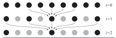
**Figure 32-6.** Three iterations of one-dimensional stationary wavelet transform while the kernel footprint increases exponentially. Arrows show the nonzero pixels of previous result contributing to the current result, while the gray dots are pixels with zero value. Figure after Dammertz et al. [2].
