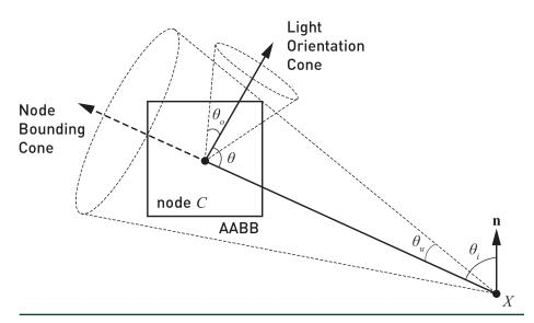
**Figure 18-3.** Description of the geometry used for computing the importance of a child node *C* as seen from a shading point *X*. In Figure 18-1, the importance is computed twice at each step in the traversal, once for each child. The angle  $\theta_u$  and the axis from *X* to the center of the AABB represent the smallest bounding cone containing the whole node and are used to compute conservative lower bounds on  $\theta_i$  and  $\theta$ .
