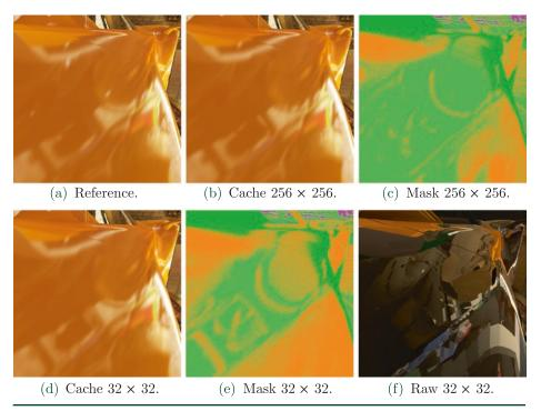
**Figure 32-12.** Reference compared to our technique when  $\alpha = 0.1$  with two different cache sizes. Note how cache hits are greatly increased by our sampling heuristics compared to Figure 32-11. Even cache size  $32 \times 32$  produces lots of cache hits for rougher surfaces but naturally less than size  $256 \times 256$ . The last image shows reflection sampling from the cache with heuristics disabled.
