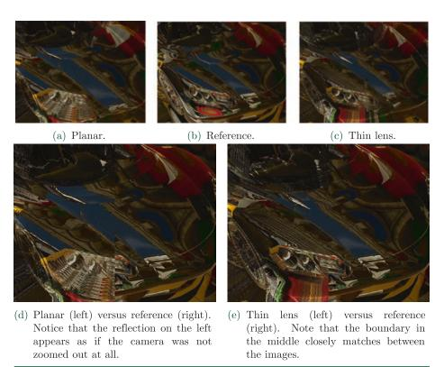
**Figure 32-9.** Comparison between view-dependent velocity vectors with the assumed planar reflector and the thin lens approximation. The camera is zoomed out approximately 1 meter during 10 frames while sampling only the previous frame's data from the screen, using coordinates offset with the motion vectors. Reflections are calculated only for the first frame.
