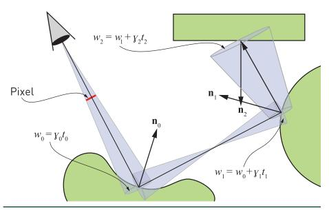
**Figure 20-3.** Illustration of how a cone is created through a pixel and how it is transported through the scene, growing and shrinking. Assuming that the rectangle is textured and the other objects are perfectly reflective, we will perform a texture lookup at the hit point on the rectangle using the width of the cone and the normal there, and a textured reflection would appear in the leftmost object. Computation of the cone widths w<sub>i</sub> is explained in the text.
