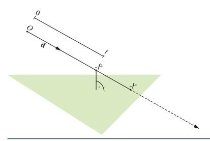
**Figure 6-1.** Calculating the ray/surface intersection point X by inserting the intersection distance t into the ray equation. In this case, any error introduced through insufficient precision for t will mostly shift the computed intersection point  $\tilde{X}$  along the ray direction **d**—and, typically, away from the plane of the triangle.
