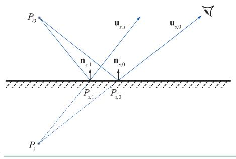
Figure 32-7. Mirror reflections in a plane.
