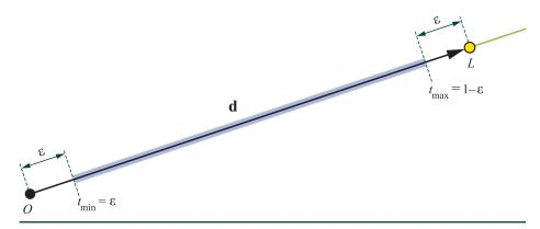
**Figure 2-3.** In this example there is a light source at L and we want to search for intersections between only 0 and L. A ray interval  $[t_{min}, t_{max}]$  is used to limit the search for intersections for t-values to  $[t_{min}, t_{max}]$ . To avoid precision problems, this restriction is implemented by setting the ray interval to  $[\varepsilon, 1 - \varepsilon]$ , giving the interval shown in light blue in this illustration.
