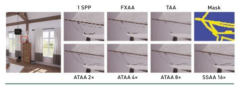
**Figure 22-1.** The Modern House scene in Unreal Engine 4 with deferred shading, ray traced shadows, our Adaptive Temporal Antialiasing technique, and a moving camera all rendered in 9.8 ms on an NVIDIA GeForce 2080 Ti. The zoomed-in inlays compare boat rope details rendered with one-sampleper-pixel (1 SPP) rasterization, FXAA, UE4's stock TAA, a visualization of our segmentation mask, ATAA 2x, 4x, and 8x, and an SSAA 16x reference.
