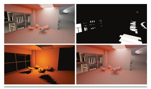
**Figure 23-13.** Visualization of the irradiance caches on the Granary scene, lit by local lights, a direction light, and a sky dome. Top left: indirect lighting stored into a light map. Top right: the directional light irradiance cache. Bottom left: the local light irradiance cache. Bottom right: red dots showing where the irradiance cache is computed.
