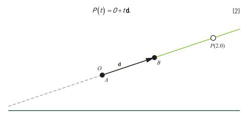
**Figure 2-2.** A ray P(t) = 0 + t d, described by an origin 0 and a ray direction d, which in this case is d = B - A. We often are interested in only positive intersections, i.e., where the points found are in front of the origin (t > 0). We depict this limitation by drawing the line as dashed behind the origin.
