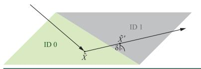
**Figure 6-4.** Rejection with primitive IDs also fails on flat or slightly convex geometry for intersections anywhere on the primitive if the next ray exists at a grazing angle. Again, the distance  $\delta$  of the false intersection  $\tilde{X}'$  to the surface of the other primitive gets arbitrarily close to zero, the primitive IDs mismatch, and hence this false intersection is considered valid.
