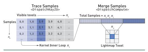
**Figure 23-8.** Left: dispatching strategy for the tracing kernel. Right: samples stored in one large buffer being accumulated and merged into a single light map texel.
