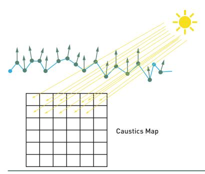
**Figure 14-9.** The water mesh is rendered to a caustics map as seen from the point of view of the light—the pixels of the resulting surface carry the position of the water surface and the normal of the water surface in this pixel.
