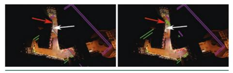
**Figure 18-7.** Visualization of the second level of the BVH when built using SAH (left) and SAOH (right); the AABB of the left child is colored in green whereas the one of the right child is in magenta. In both cases, 16 bins were used and all three axes were considered.
