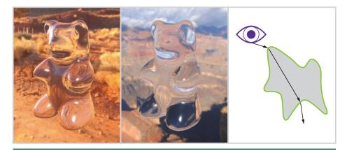
Figure 25-19. Object-space ray traced smooth transparency.
