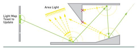
**Figure 23-6.** Irradiance evaluation of a texel. For this purpose, a path is constructed in green. At each vertex of this path, the direct lighting is evaluated by casting rays toward the area light (a.k.a. next event estimation). The number of samples for each light is proportional to its subtended solid angle. If no geometry is intersected, the sky dome radiance is evaluated.
