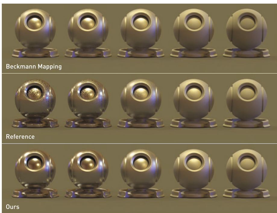
Figure 12-6. Roughness expansion of a GGX material according to a filtered antialiased normal distribution using a common Beckmann variance mapping (top) and using our GGX's variance approximation (bottom), both compared to a non-filtered reference (middle). In this test case, the GGX base surface roughness is varying from 0.01 (left) to 0.8 (right) and shows that our approximation better preserves the overall perceived roughness induced by the underlying normal distributions.
