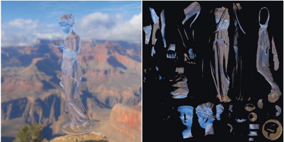
Figure 25-22. Object-space ray traced transparency: result (left) and texture-space output (right).
