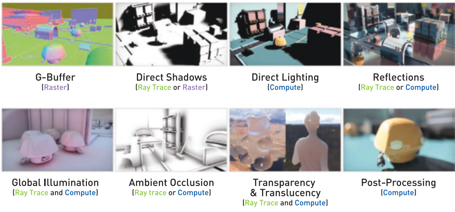
Figure 25-2. Hybrid rendering pipeline.
