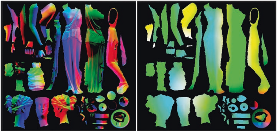
Figure 25-21. Object-space parameterization: normals (left) and positions (right).
