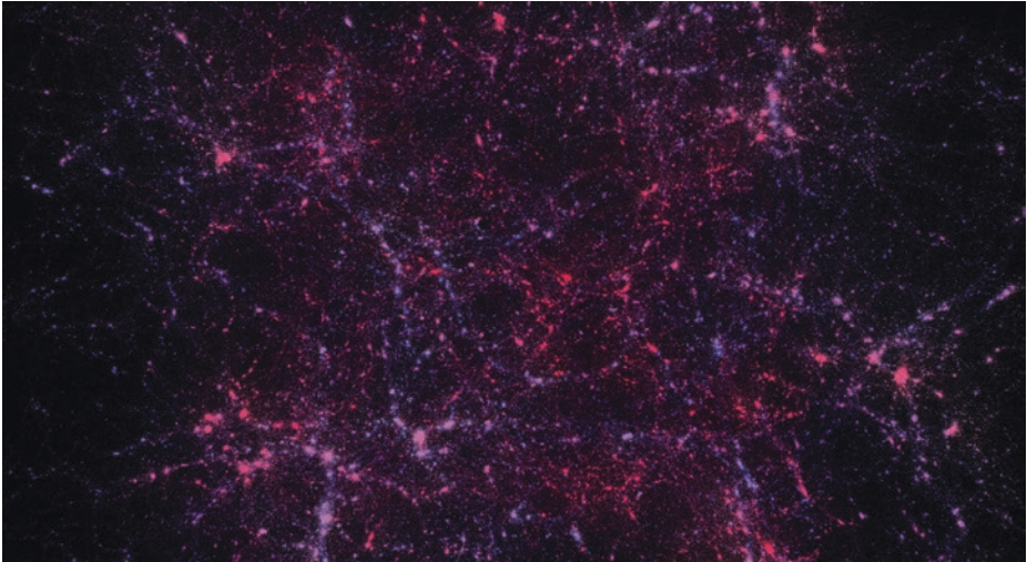
Figure 29-1. One hundred million particle subset of the DarkSky N-body gravitational cosmology simulation, rendered in its entirety at 35 FPS (1080p) or 14 FPS (4k) without level of detail, on an NVIDIA RTX 2080 Ti with RT Cores technology.
