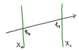
In 3D, those boundaries are planes. The equations for the planes are x = x0, and x = x1. Where does the ray hit that plane? Recall that the ray can be thought of as just a function that given a *t* returns a location p(t):
