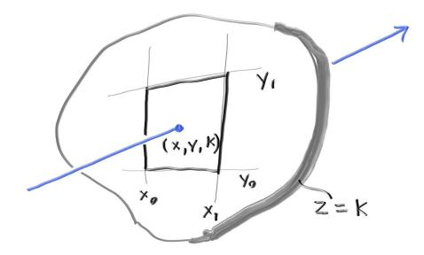
To determine whether a ray hits such a rectangle, we first determine where the ray hits the plane. Recall that a ray  $p(t) = a + t^*b$  has its *z* component defined by  $z(t) = az + t^*bz$ . Rearranging those terms we can solve for what the *t* is where z=k.
