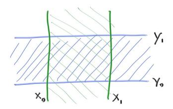
For a ray to hit one interval we first need to figure out whether the ray hits the boundaries. For example, again in 2D, this is the ray parameters t0 and t1. (If the ray is parallel to the plane those will be undefined.)
